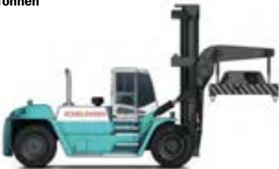
Standardkabine 3–4 hoch 33–35 Tonnen
